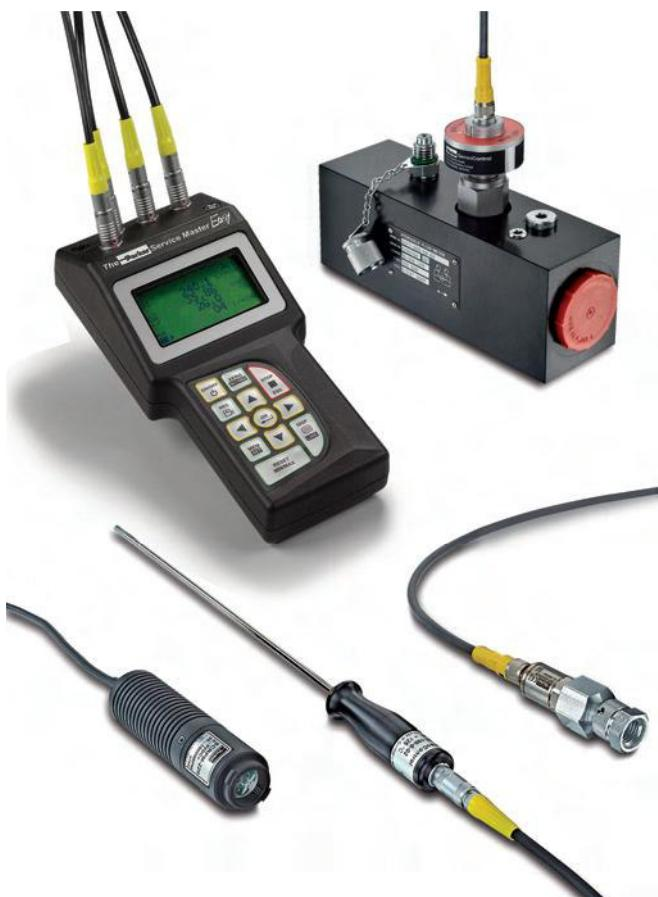
**The Parker Service Master Easy** is a multi-channel handheld measuring device for the simultaneous measuring of important hydraulic values.
