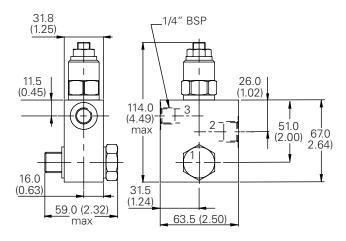
Complete Valve - Dual Overcenter 3/8" Ports Basic Code 1CEE35/1CEEB35/1CEER35/1CEEL35 (Internally Cross-Piloted)
