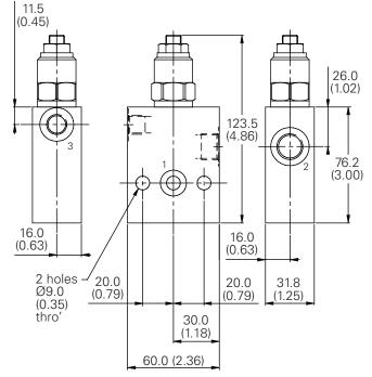
Note: Tightening torque of "F" adjuster locknut= 20-25 Nm.
