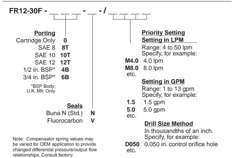
Note: Minimum drill diameter is 0.020 in. For smaller orifice sizes consult factory.
