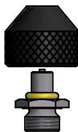
Model of valve stem 7/8" 14 UNF (B)
