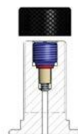
Model of valve stem integrated 5/8" 18 UNF (D)
