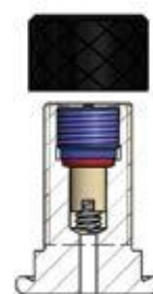
Model of valve stem integrated 7/8" 14 UNF (C)
