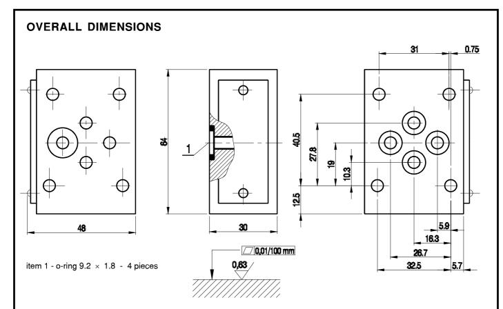
Admissible surface roughness and flatness deviation for a subplate face.
