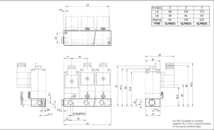
P.S.: Base is supplied complete with plug, tubing and junction seals.
