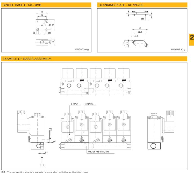
P.S.: The connection nipple is supplied as standard with the multi-station base
