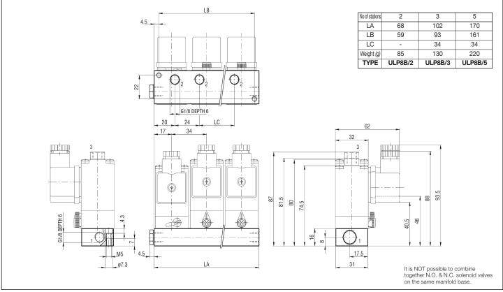
P.S.: Base is supplied complete with plug, tubing and junction seals.
