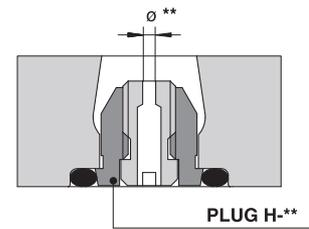
**13 ELECTRIC CONNECTORS ACCORDING TO DIN 43650** (to be ordered separately)
