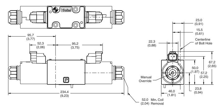
Note: 22.0 mm (0.87") from bottom of bolt hole counterbore to bottom of valve.
