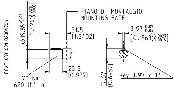
**STRAIGHT****50**Mounting face refer to flange code **S1****○**
