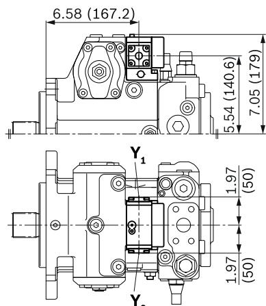
▼ HW – Proportional control, hydraulic, mechanical servo
