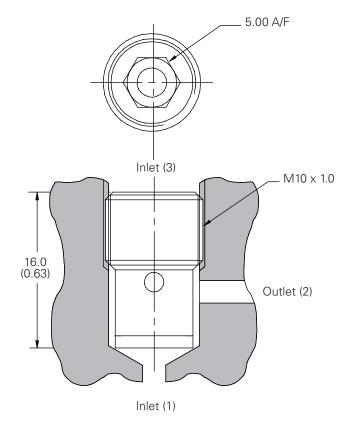
Note: Using LOC-TITE 542, torque cartridge to 8-10 Nm against the bottom of the cavity.
