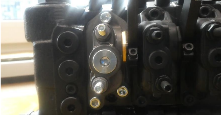
4-3: Assembling of CH Cap A-Side (Lever Housing)
