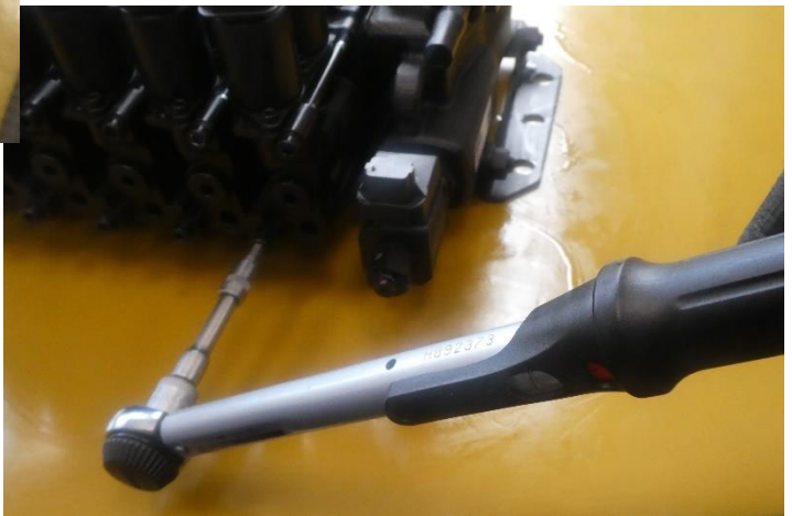
4-4: Assembling of Electrohydraulic Spool Actuator, B-Side
