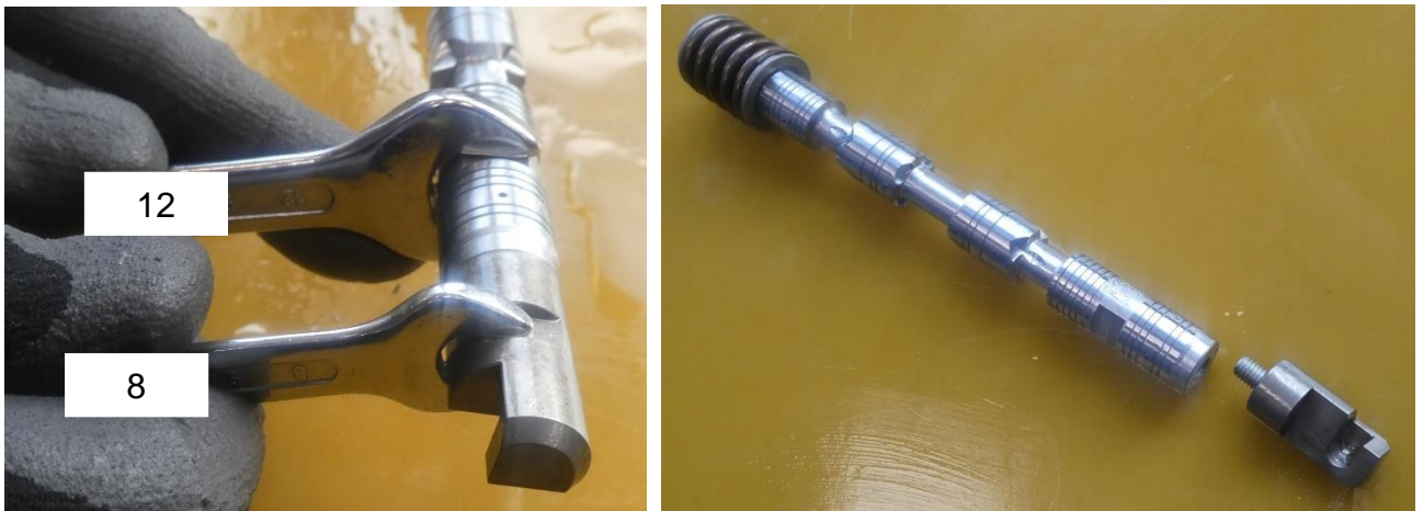
3-4: Disassembling of Spool End Tap
