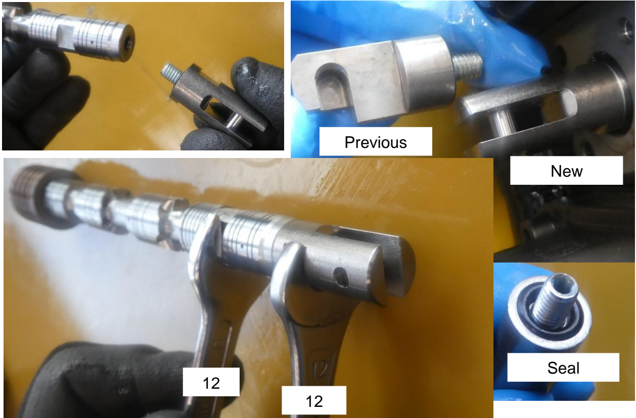
4-2: Assembling of New Spool End Tap
